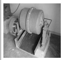
Figure 3: A sample ball mill.
