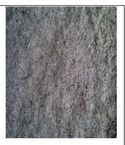
Figure 2: RHA after combustion
